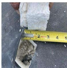
**Roof System Notes:** Two (2) test core samples were taken at the roof drain (low point 2.5") and the roof system's perimeter (high point 2.5").
