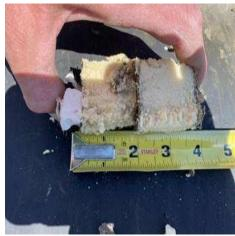
**Roof System Notes:** Two (2) test core samples were taken at the roof drain (low point, 3.5") and the roof system's perimeter (high point, 3.5").
