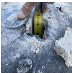
**Roof System Notes:** Two (2) test core samples were taken at the roof drain (low point, 2.5") and the roof system's perimeter (high point, 7.5").
