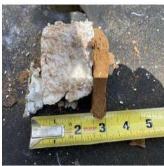
Roof System Notes: Two (2) test core samples were taken at the roof drain (low point 3.0") and the roof system's perimeter (high point 3.0").
