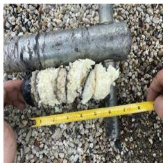
**Roof System Notes:** Two (2) test core samples were taken at the roof drain (low point 3.5") and the roof system's perimeter (high point 10.0").
