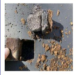
**Roof System Notes:** Two (2) test core samples were taken at the roof drain (low point 3.0") and the roof system's perimeter (high point 4.5").
