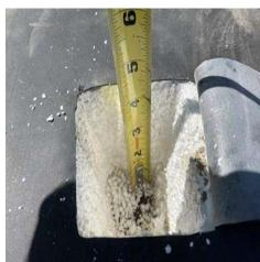
**Roof System Notes:** Two (2) test core samples were taken at the roof drain (low point 4.0") and the roof system's perimeter (high point 4.0").
