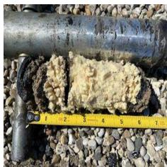
**Roof System Notes:** Two (2) test core samples were taken at the roof drain (low point, 3.0") and the roof system's perimeter (high point, 7.0").
